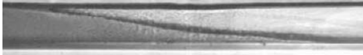
FIGURE 1. The dark fluid is the sugar solution that has become denser because of downward diffusion of salt from the overlying salt solution. The slanting interface is nearly linear and the fronts penetrate laterally with nearly constant velocity.
